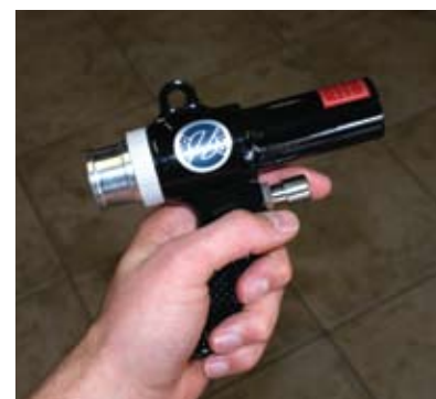
Ready, aim, fire: A blow/vac or air venturi gun is the best applicator for inert dust.
